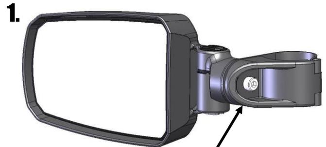
Temporarily remove this socket head bolt using a 8mm Allen Wrench
