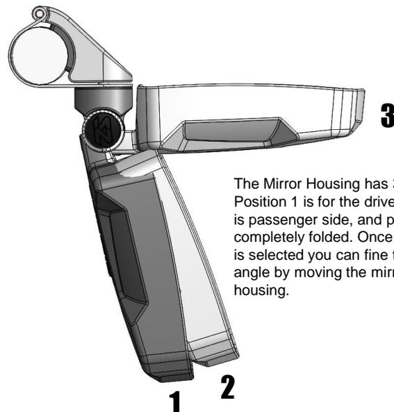
The Mirror Housing has 3 detent positions. Position 1 is for the drivers side, position 2 is passenger side, and position 3 is completely folded. Once the detent position is selected you can fine tune the viewing angle by moving the mirror glass within the housing.
