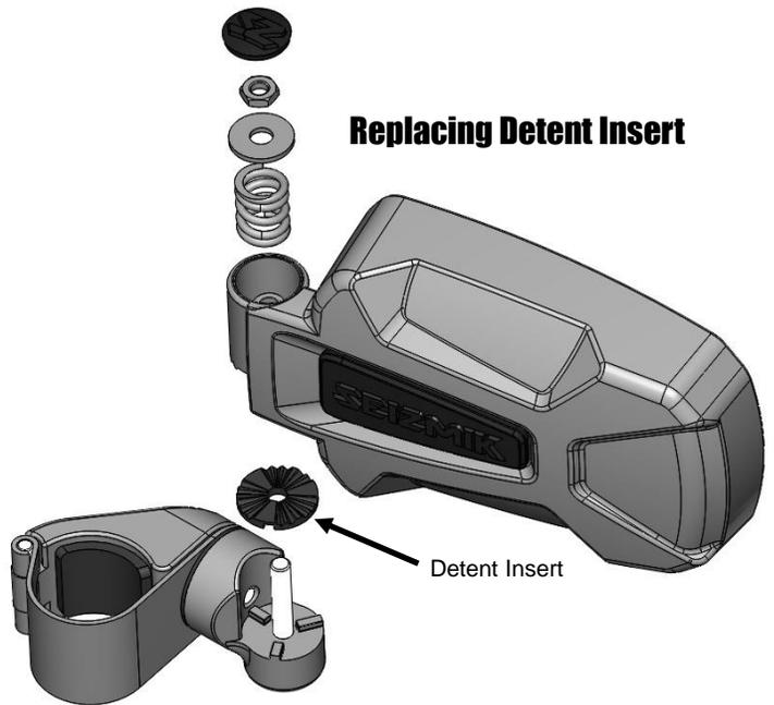
If for any reason the Mirror Detent Insert ever becomes worn enough that the mirror will not hold position well, please contact us for free replacements. It can be replaced by first removing the nut shown in the previous step. Next, remove the Mirror Housing, Spring, and Washer. The Detent Insert can now be gently pried off and replaced. The detent is designed so it can only go on one way.
