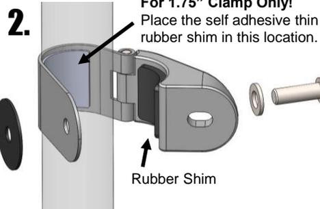
Open clamp and place around roll cage tube. Make sure the rubber shim is in place in the thick half of the clamp.
