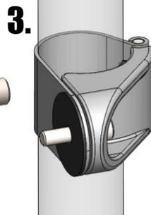
Close clamp around roll cage tube, put the bolt through the hole, and place large rubber washer over the end of the bolt.
