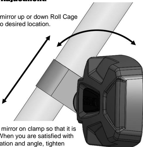
Rotate mirror on clamp so that it is level. When you are satisfied with the location and angle, tighten bolt.
