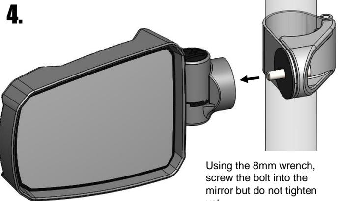
Using the 8mm wrench, screw the bolt into the mirror but do not tighten yet.
