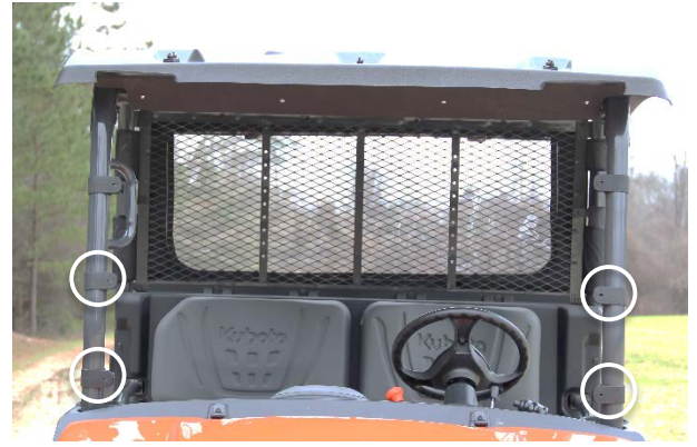
6. Place four clamps in the approximate locations shown.
