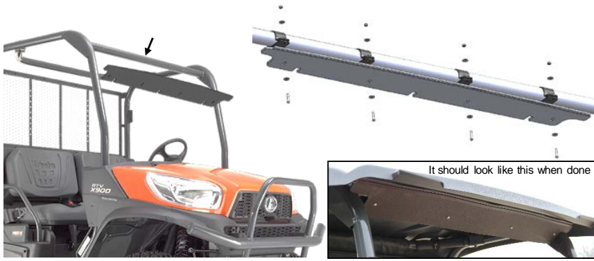
5. Bolt the Header panel in front of the upper cross bar in on the RTV X with 4 plastic p clamp bolts and washers.
