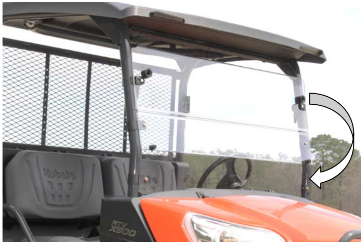
16. Push the top half of the windshield down and firmly press the two rubber plugs against each other to lock windshield in down position.
