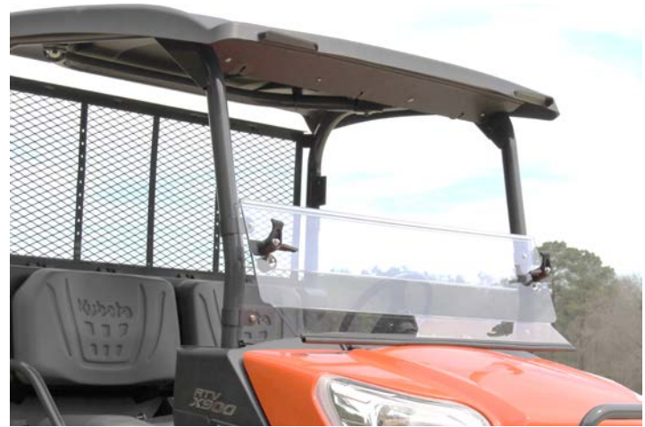
16. Push the top half of the windshield down and firmly press the two rubber plugs against each other to lock windshield in down position.
